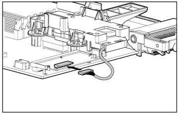
Figure 1-20: Cabling the Battery-Backed Write Cache Enabler
